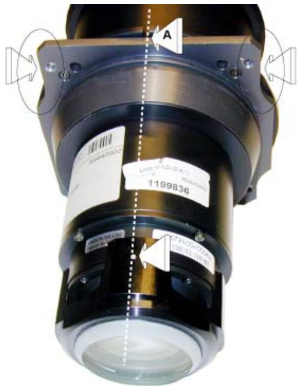
Image 2-2 Lens adapter lining up
